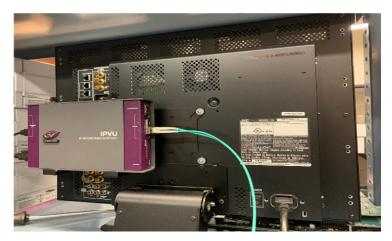
Figure 3: Zero Rackspace IPVU using Vesa-Mounting Kit
